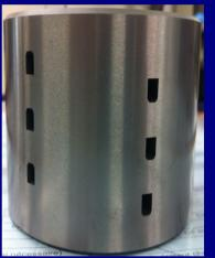
No microcracks due to erosion
